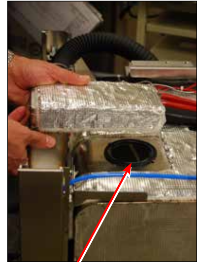
Figure 44d condenser gasket
