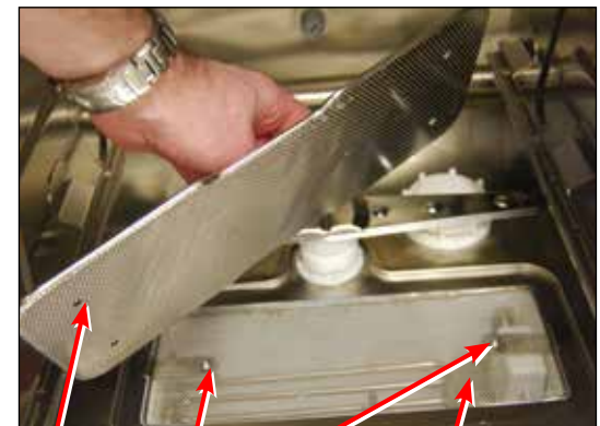
coarse filter fine filter screws fine filter Figure 7
